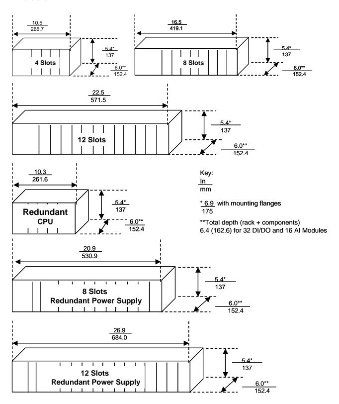
Figure 2 HC900 Process Controller Dimensions
