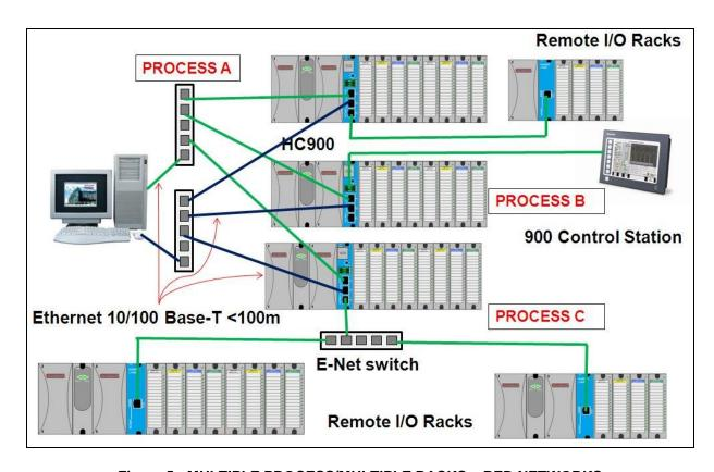
Figure 5 - MULTIPLE PROCESS/MULTIPLE RACKS - RED NETWORKS
