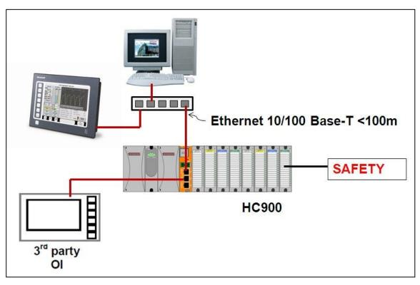
Figure 2 - SINGLE PROCESS/SINGLE RACK- SAFETY
