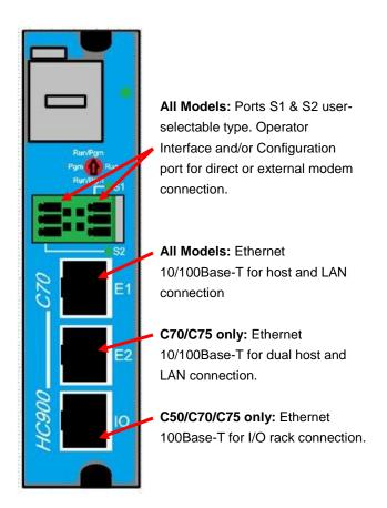
**Figure 1 Communication ports**
