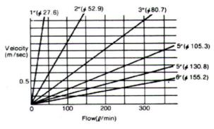
Calculate: O(Flow)=D2/4×V×10-2(L/min) V(Velocity)=m/sec D=Inner diameter of pipe(mm)
