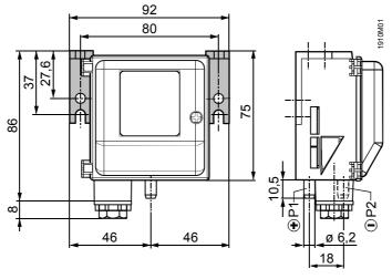
Air duct probe (ABS)
