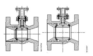
Special taper shape in inlet part of ball valve provides the ball valve control with excellent control capability.
