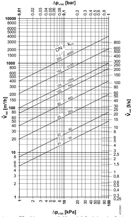
$\Delta p_{v100}$  = Differential pressure across the fully open butterfly valve by a volume flow  $\dot{v}_{100}$
