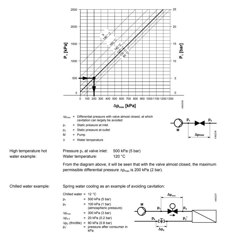
Working pressure and medium temperature Fluids
