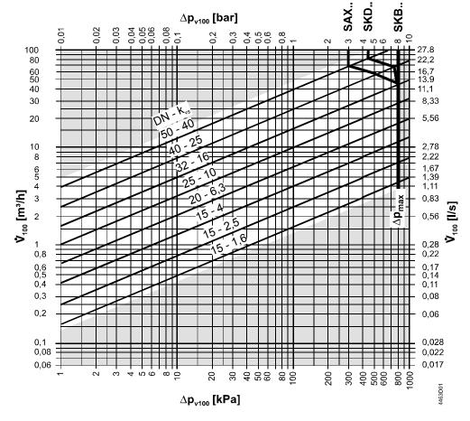
$\Delta p_{\text{max}}$  = Maximum permissible differential pressure across the valve (mixing: port A - AB, B - AB), valid for the entire actuating range of the motorized valve
