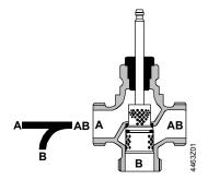
Guided perforated plug which is integrated in the valve stem.
