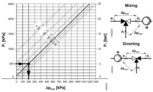
$\Delta p_{\text{max}}$  = Differential pressure with valve almost closed, at which cavitation can largely be
