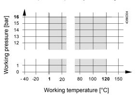
Working pressure and medium temperature staged as per ISO 7005
