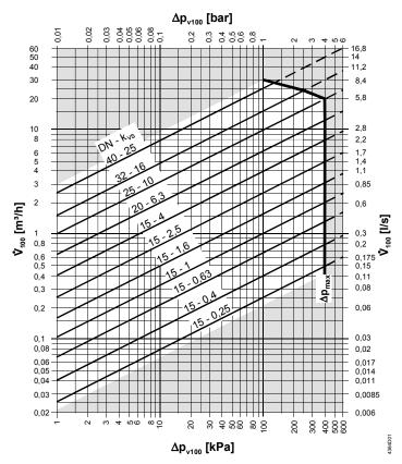
$\Delta p_{max}$  = Maximum permissible differential pressure across the valve (mixing: port A - AB, B - AB), valid for the entire actuating range of the motorized valve
